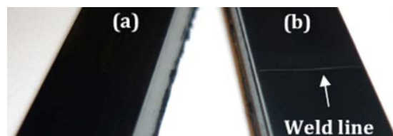
Figure 8. Comparison of specimens produced (a) employing the RHCM system and (b) by conventional injection molding. 54 [Color figure can be viewed in the online issue, which is available at wileyonlinelibrary.com .]
